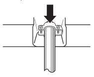
3. Install power supply cord strain relief.
