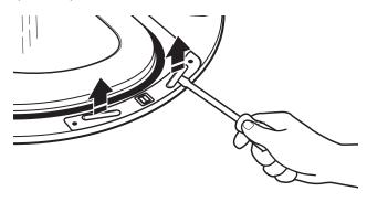
2. Remove the four screws that attach to inner door hinge.
