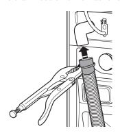
3. Once the drain hose is in place, release the pliers.
