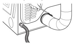
Make sure the vent is secured to exhaust hood with a 4" (102 mm) clamp.
