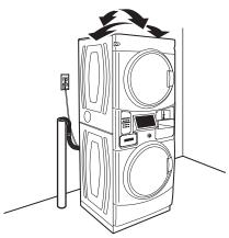
3. If washer/dryer is not level, use a 9/16" or 14 mm open-end or adjustable wrench to turn jam nuts clockwise (as viewed from above) on feet until they are about 1/2" (13 mm) from the washer/dryer cabinet. Then turn the leveling foot counterclockwise to lower the washer/dryer or clockwise
