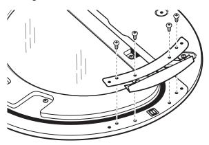
4. Reinstall plug strips on opposite side of the inner door.
