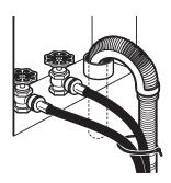
The top of the standpipe must be at least 30" (762 mm) high and no higher than 96" (2.4 m) from the bottom of the washer.
