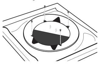
6. Lift and rotate center insert 180 degrees.
