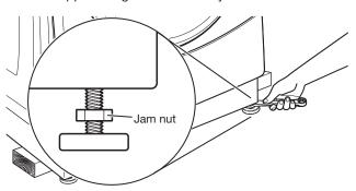
4. When washer/dryer is level and all four feet are firmly in contact with the floor, use a 9/16" or 14 mm open-end or adjustable wrench to turn jam nuts counterclockwise (as viewed from above) on leveling feet tightly against washer/ dryer cabinet.
