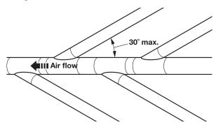
The maximum angle of each vent entering the main vent should be no more than 30.°
