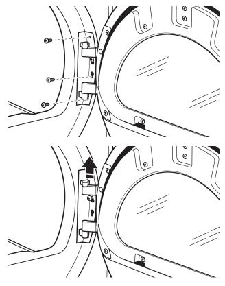
3. Lay the door assembly on a previously prepared flat surface with the inside (inner door assembly) facing up, and remove six Phillips head screws to release outer door assembly from inner door assembly.
