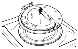
**5.** Remove four Phillips head screws to release center insert from outer door ring.
