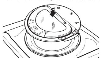
2. Reassemble the inner and outer door assemblies with the six screws.
