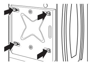
3. Once the bolt is loose, move it to the center of the hole and completely pull out the bolt, including the plastic spacer covering the bolt. Once all four bolts are removed, discard the bolts and spacers.
