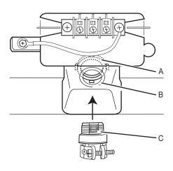
Put direct wire cable through the strain relief. The strain relief should have a tight fit with the dryer cabinet and be in a horizontal position. Tighten strain relief screw against the direct wire cable.
