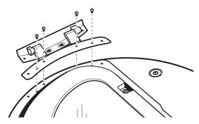
3. Move hinge to other side. Reinstall four screws.
