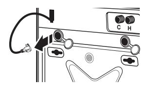
**5.** Close the bolt holes with the four transport bolt hole plugs.
