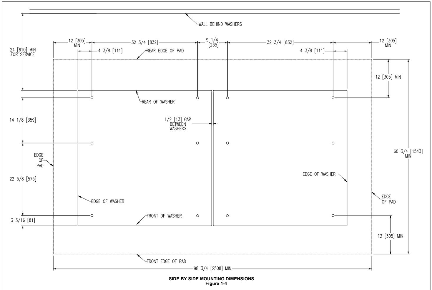
*2.7.17 T-1450/1475 Machine Side By Side Mounting Detail*
