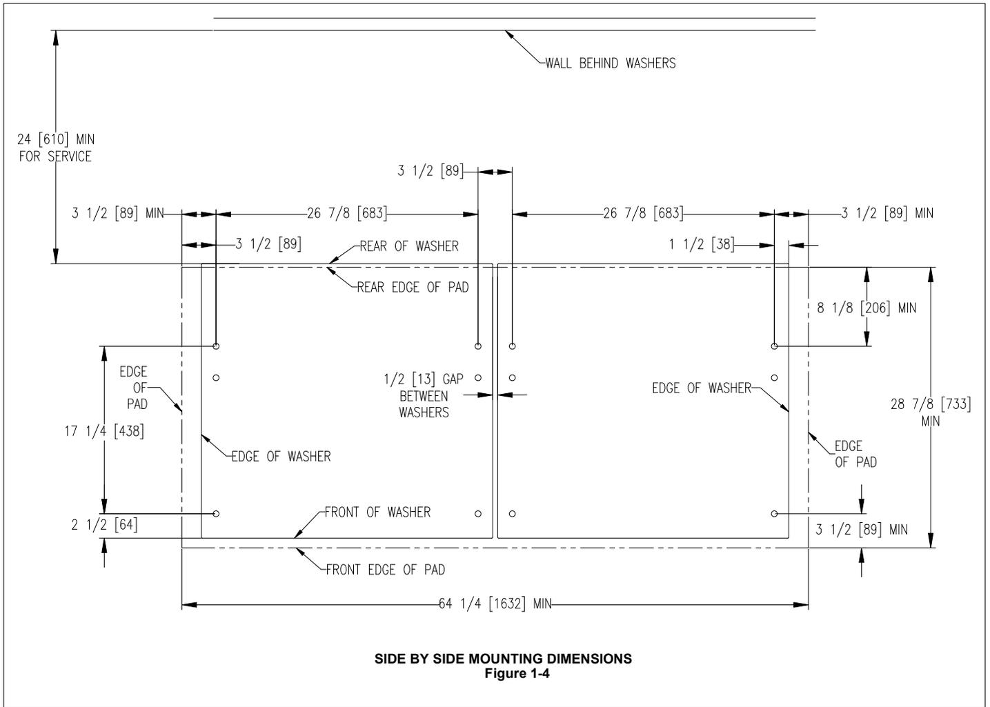
*2.7.5 T-450 Machine Side by Side Mounting Detail*
