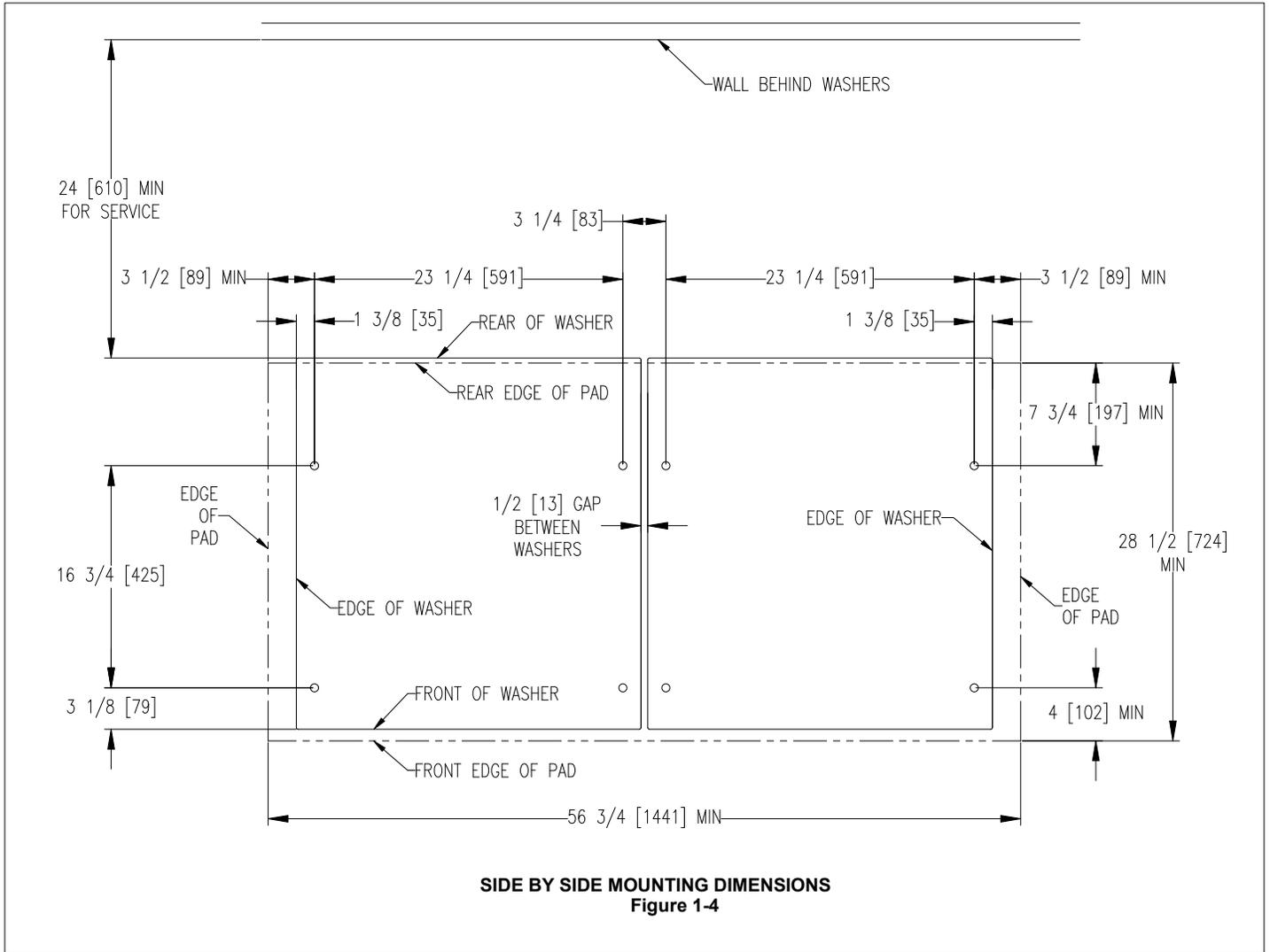
*2.7.2 T-350 Machine Side By Side Mounting Detail*
