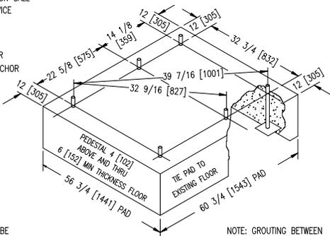
PEDESTAL SHOULD BE 4,000 PSI [28 MPa] MIN CONCRETE REINFORCED WITH MESH OR RODS.
