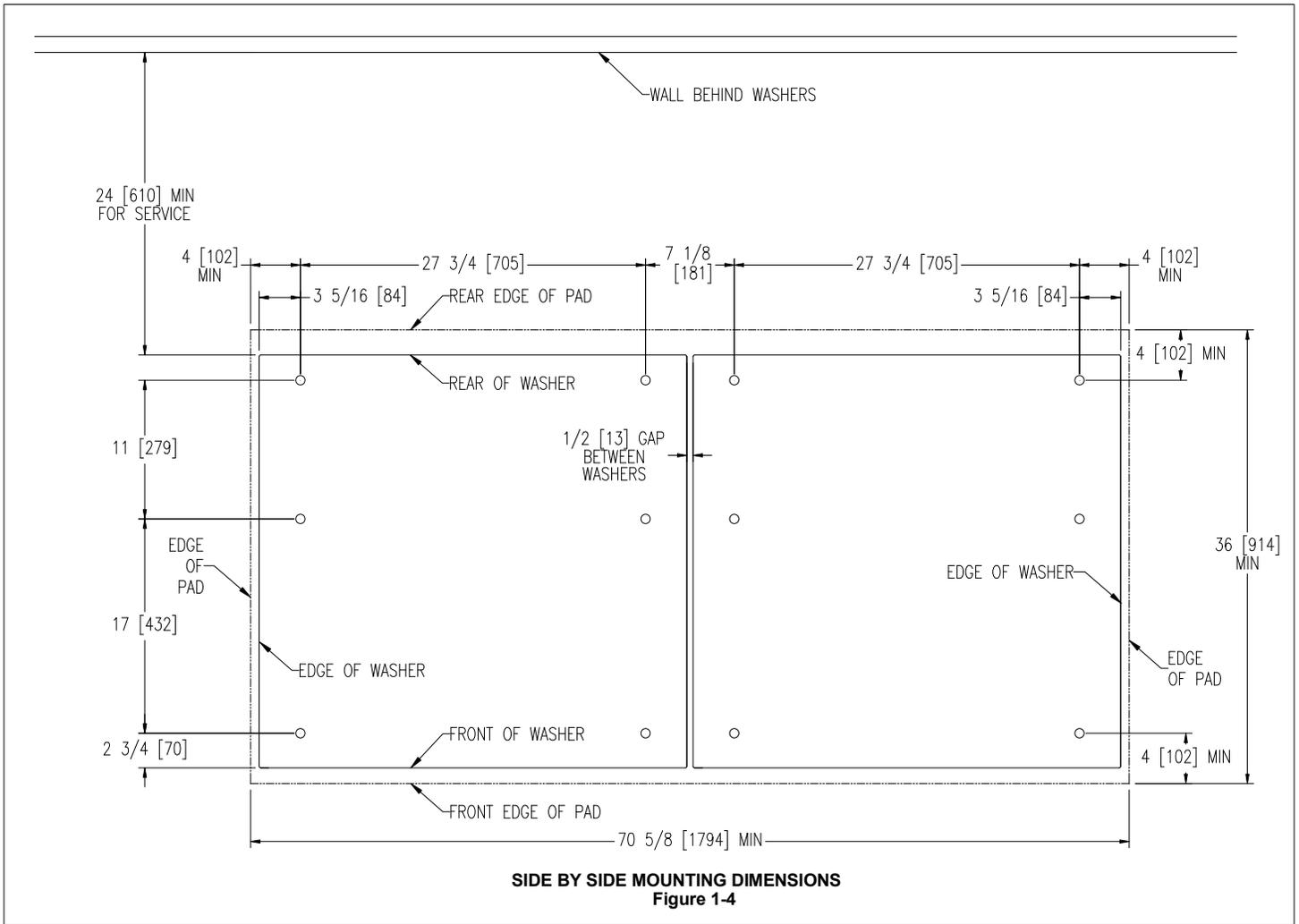
*2.7.11 T-750 Machine Side By Side Mounting Detail*
