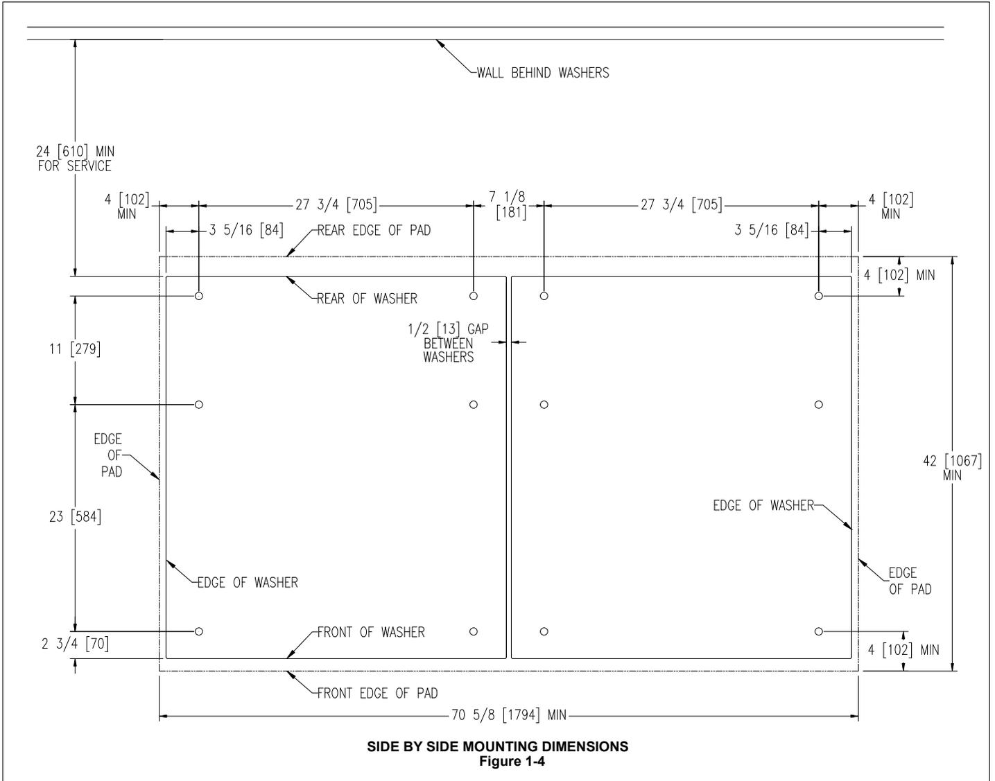
*2.7.14 T-950/975 Machine Side By Side Mounting Detail*
