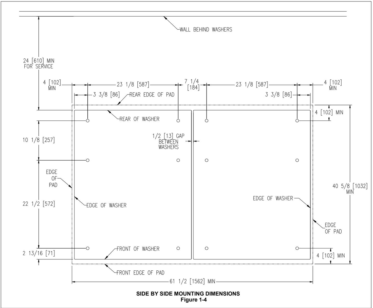
*2.7.8 T-650/675 Machine Side By Side Mounting Detail*
