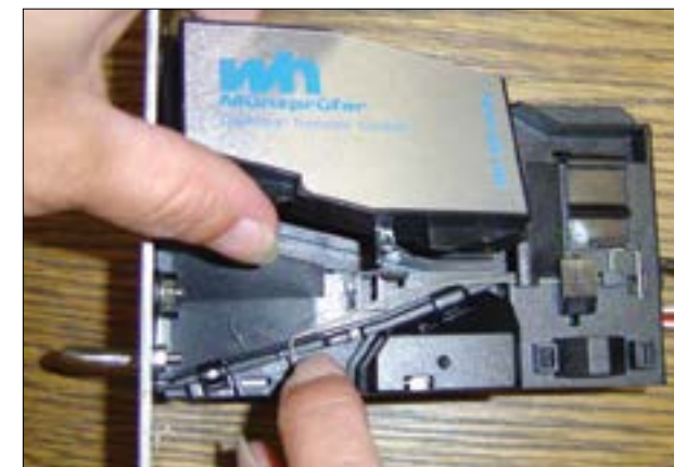
Open the flap of the coin selector.
