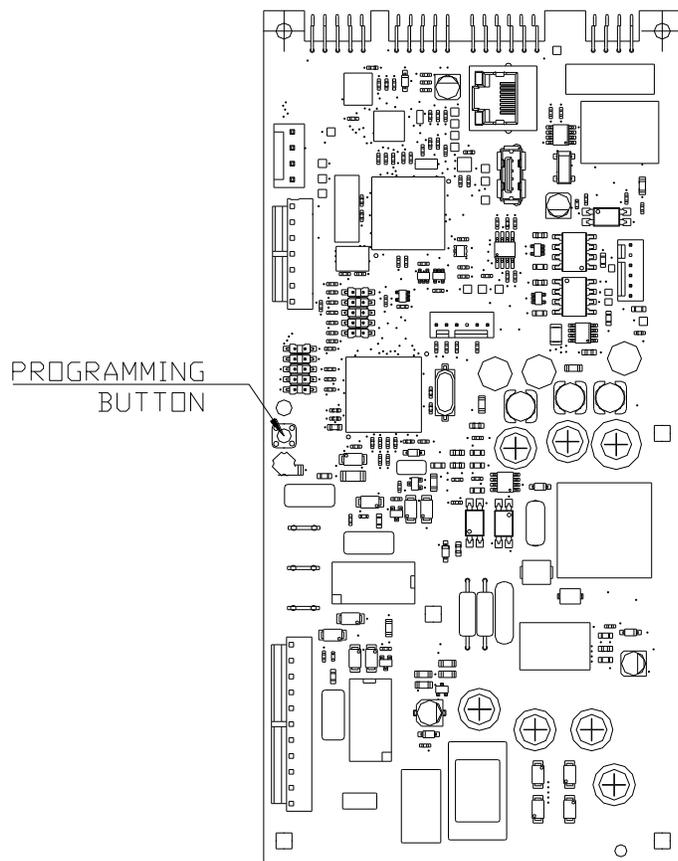
When manual programming mode is entered, the "Start", "High", "Medium" and "Low" buttons perform alternate functions.
